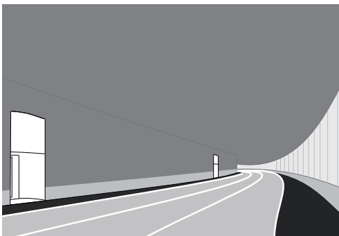
Bergtunnel - asymmetrisk materialkomposition.
