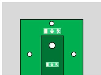
*Figure 6. Recommended colour scheme of the portal.*
