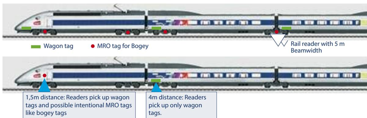
\* Current empiric tests have shown that trackside reader systems can cope with 3 visible tags on a 5 m segment of trains up to 160 km/h and with only 1 visible GIAI-96 tag on a 5 m segment of train at speeds of 200 km/h.
