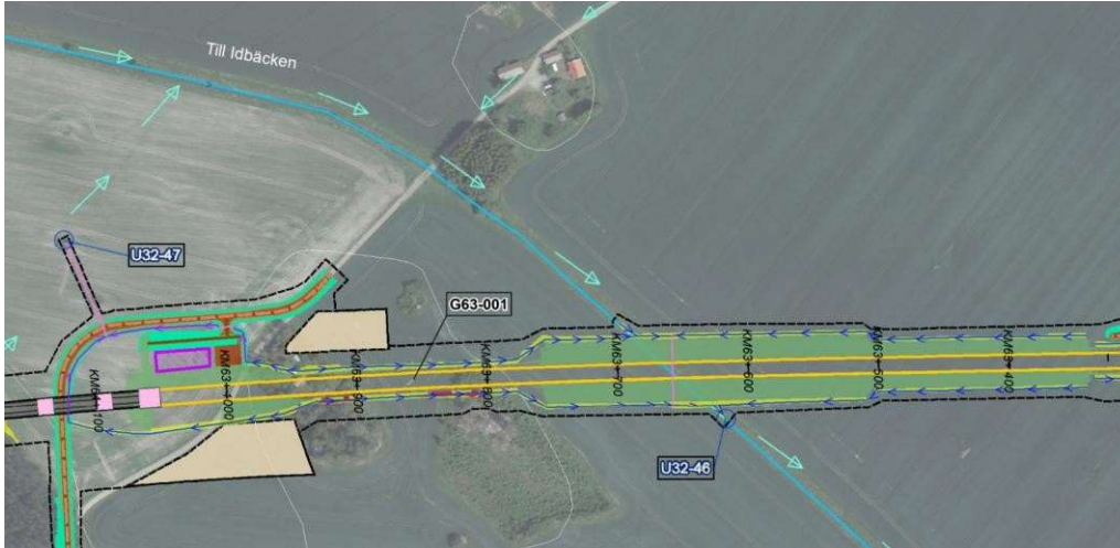
Figure C1.10. Discharge points within the Ålberga contract to the land drainage contractor Jordbron–Djelp tf.
