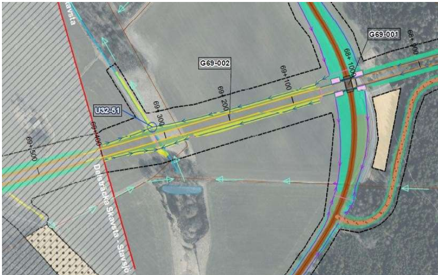
Figure Ci.14. Discharge point to the Vik-Rällinge TF land drainage system (ID 404).
