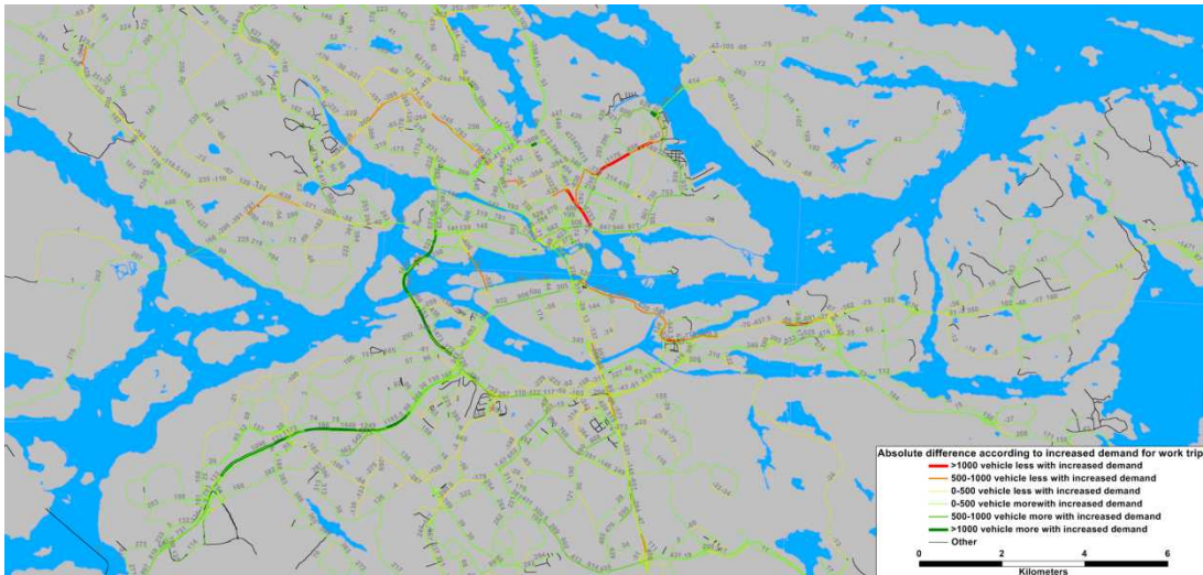
Figure 30: Absolute flow difference between 7 and 8h with regards to increased work trips demand
