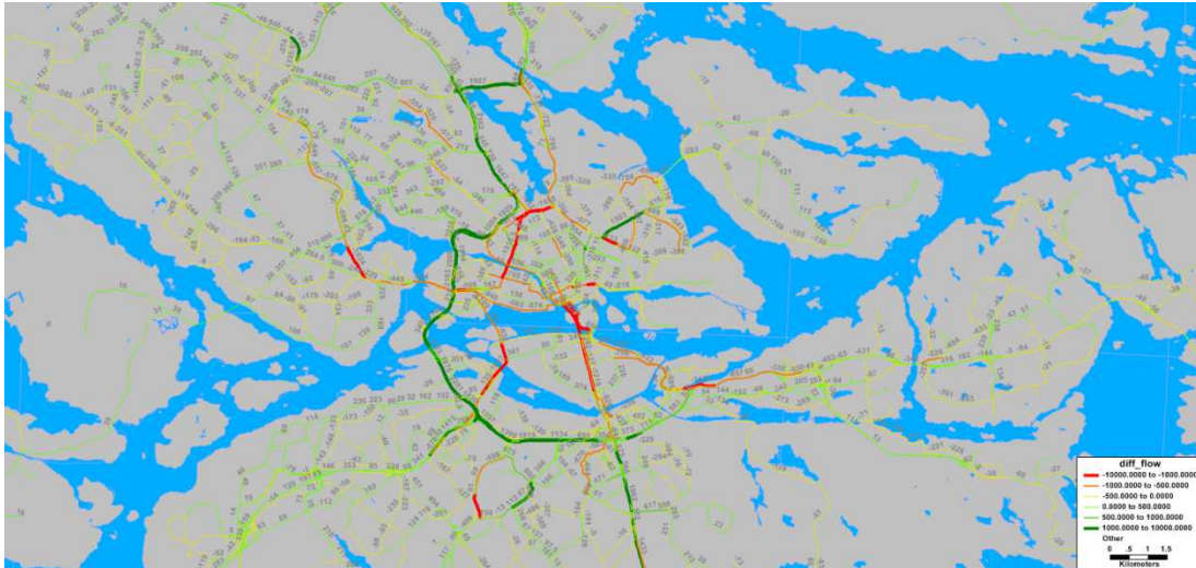
Figure 24: Effect of congestion charge on traffic in morning peak hour (7-8h); Red = more without congestion charge, Green = more with congestion charge
