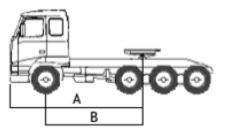
In an application for transport exemption measurement (**B**), working distance front axle to centre of connector, must be indicated. This can be obtained by subtracting the vehicle's forward overhang from measurement (**A**).
