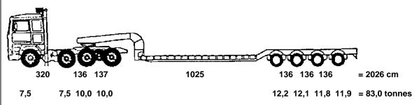
Remember to indicate the centre of gravity of the load measured from the trailer's/semi-trailer's front axle when transporting heavy loads!
