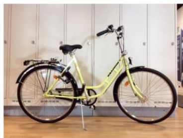
Fig 3. Instrumented bicycle: 9-dof IMU on the rear frame, steer angle potentiometer, DC generator for forward speed measurement, and a Raspberry Pi 3 for data logging. City bicycle with step-through frame, a coaster brake at the rear, and a roller brake at the front.
