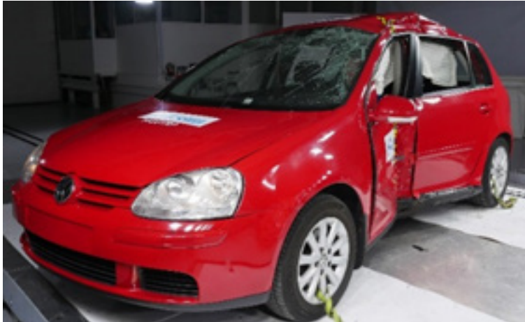
Figure 52. VW Golf (rust) pole test.
