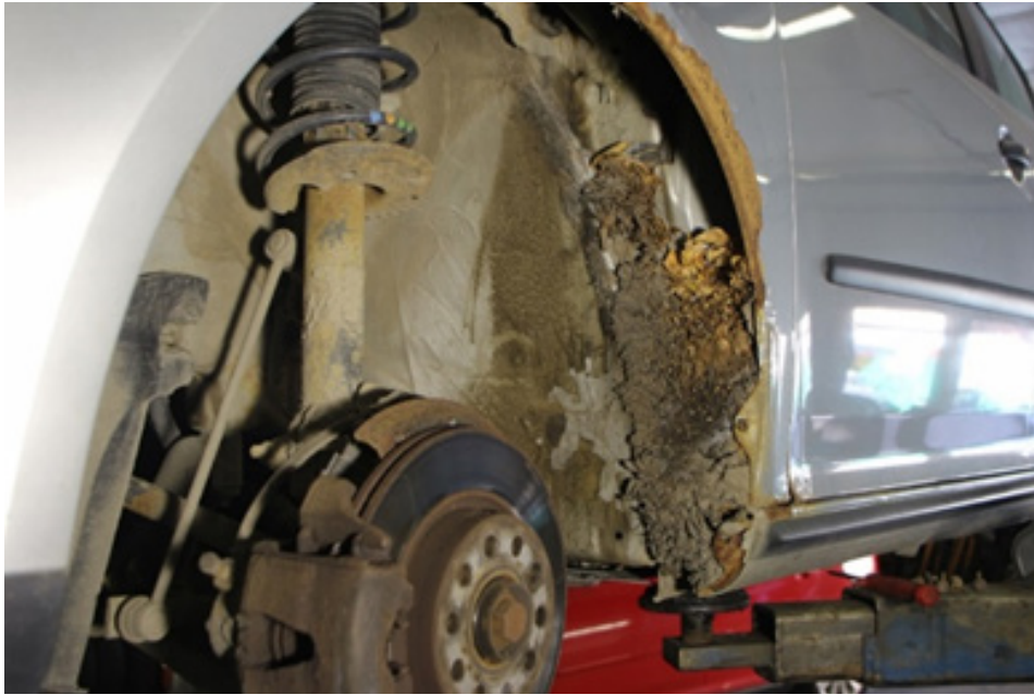
Figure 1. Dirt behind plastic inner fender.
