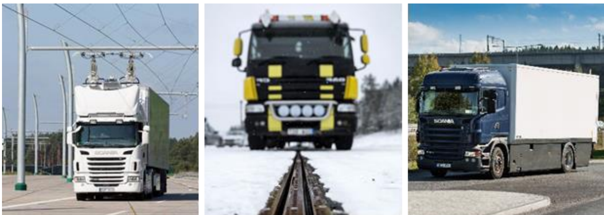
Figure 2: Example illustrations of the three transmission technologies, from left: transmission via overhead power lines [17], transmission via a rail in the road [12], transmission via electromagnetic fields [18]
