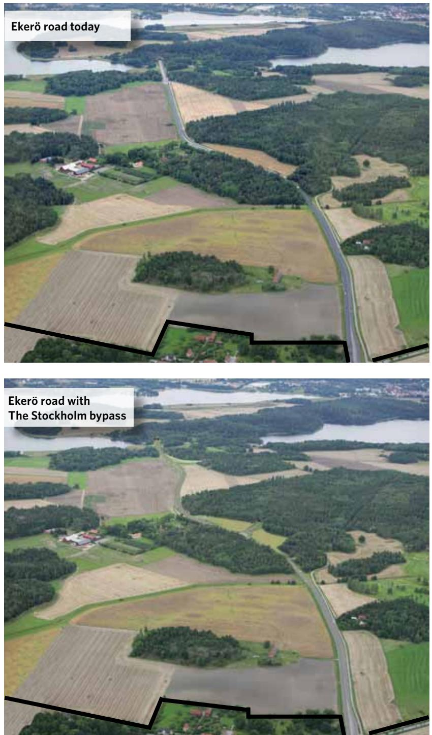
Fig 10. Stockholm Bypass junction without changes on the Ekerö Road north of Edeby. World heritage boundary shown at the bottom of the pictures. The proposed widening of the Ekerö Road is not shown.
