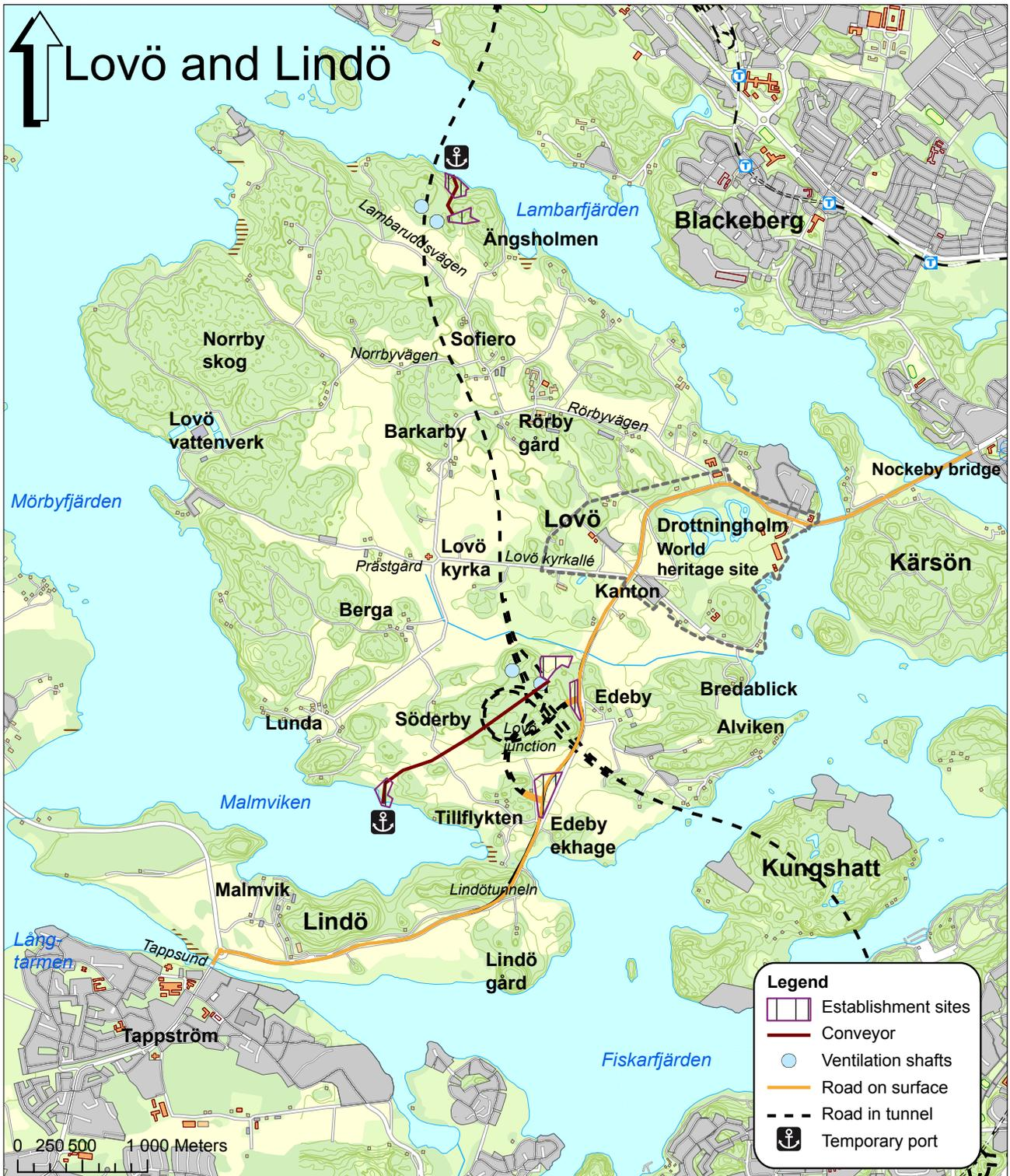
Fig 12. Establishment sites and construction work areas on Lovö
