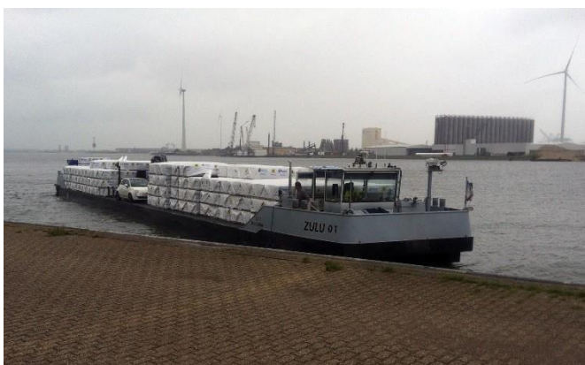
Figur 14 Pallet Shuttle Barge
